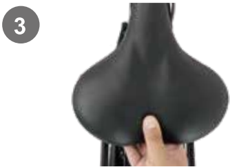
3. Adjust the seat and the head of the seat is parallel with the top tube.
